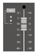
Pressing and holding the **auto** button **35** on a channel fader will display the current automation mode for that channel in the channel scribble strip display. To display the automation mode on all channels select the Status Group (**StGr**) soft menu, and press **Auto**.
