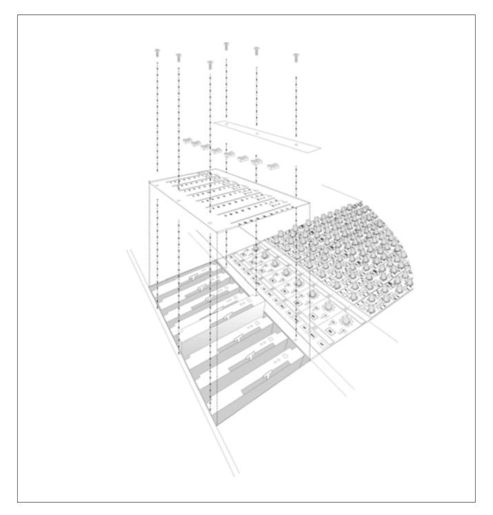
First remove all of the fader knobs from the faders in that bay. Do this by simply pulling firmly on each one until it separates from the fader tang. Then, unscrew the six countersunk screws and remove the top plate. Each fader can then be lifted clear from its connector on the bus card. When reassembling, the top plate has locating pins that locate into each fader to ensure its correct positioning.
