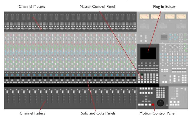
The AWS 900+ SE faders and Solos and Cuts panels can be switched between controlling the analogue audio signal path and the DAW using the Focus switch - see below. The Motion Control Panel, Master Control Panel and Plug-in Editor always control the DAW. The illustration above shows the DAW controller elements in 'DAW Focus Mode'. The greyed-out areas indicate analogue-only console elements.
