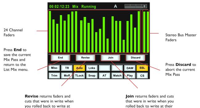
At any time you can rewind the system, and as soon as the DAW is located to an earlier time and valid MTC or a MMC locate position command is received, the mix system enters '**Mix Review**'. All faders will switch to **Replay** status (all LEDs are off). This operation is known as a **rollback**.
