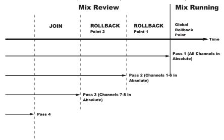
To return all faders to Absolute, operate the **Join** or **Revise** keys until the Global Rollback memory is reached, at which point all faders return to write either at the current position, via the **Revise** function, or at the balance at the Global Rollback point, via the **Join** function.
