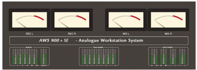
Fitted above the centre section are four VU meters dedicated to reading left and right outputs of the Record and Mix busses.
