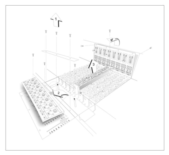
First, remove the scribble strip (three screws). Now remove the Solos and Cuts Panel (629922X1) that fits across the bottom of each bay of eight channels; remove the two countersunk screws, then carefully lift the panel clear onto a piece of foam or bubble wrap. Disconnect the ribbon and put the panel to one side.
