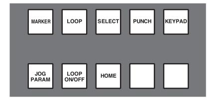
Tallies are shown in the status area of the TFT display for Loop ON/OFF, Jog Parameter, together with tallies for Marker, Loop, Select and Punch. As the later functions intercancel, they share the same on screen area.
