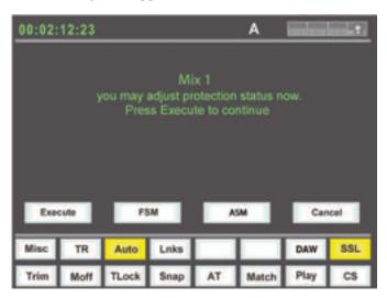
To select the different protection modes, press the **ASM** switch, and then press the fader auto switch on the desired channel to switch between modes. To globally select the mode, press the **ASM** switch then the **FSM** switch to switch between modes. The modes are displayed in the scribble strips above the faders.
