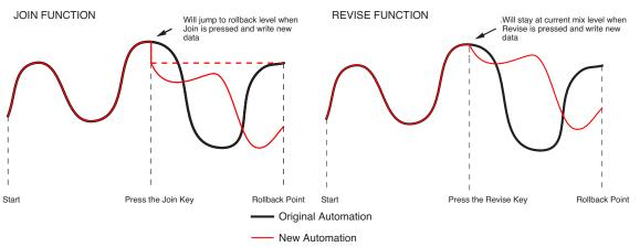
Multiple Rollback memories are supported so that successive operations of **Join** or **Revise** return different sets of faders back to the write state, if multiple Rollback operations have taken place.
