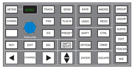
The majority of functions are controlled via dedicated keys with less reliance on the 8x8 key matrix located beneath the screen than the HUI interface.
