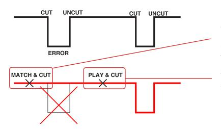
If you have made a cut error, position the DAW before the error, resume play, select Match and then press Cut to automatically drop into write without changing its current state.
