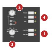
The 'Oscillator' section (see left), located above the TFT screen, contains controls for frequency, level and routing of tone or pink noise to the Mix, Record and Track bus outputs and to the monitor outputs for use in monitor calibration (see page 4-22).
