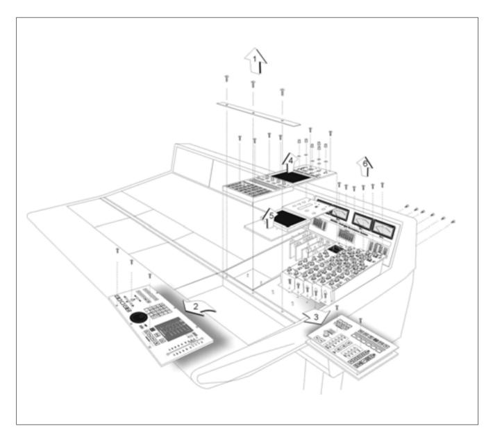
Four centre section cards are located beneath the large panel that contains the Talkback and Oscillator controls, LCD display, and DAW soft keys. These are:
