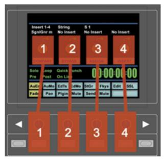
The Plug-In Editor includes an 8x8 matrix of soft buttons which map to the 16 boxes at the bottom of the plug-in display:
