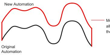
Move the fader up or down to the new value and all the existing moves will be copied exactly at the new level
